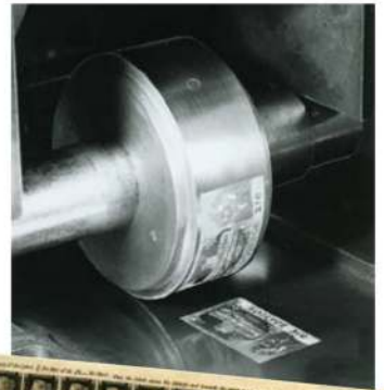
Fig 17 Creating a recess printing plate (1)—transferring an image from master die to roller (using a 1955 Castles engraving). Image copyright Royal Mail, courtesy of the BPMA
